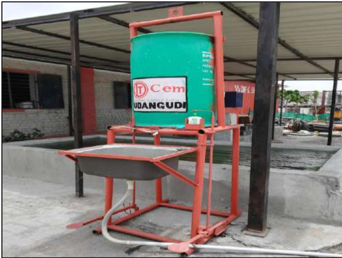
Foot Operated Hand Wash Facility at Coal Jetty Site, Udangudi (45418 DM)
